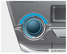
Turn the temperature control knob to the desired temperature. If the temperature is set to the lowest setting (Lo), the air conditioning system will operate continuously. To turn the automatic operation off, select any button of the following:
