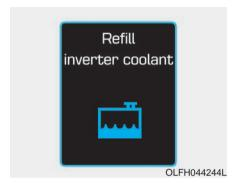
This warning message is displayed when the inverter coolant is nearly empty.
