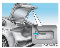
Your vehicle is equipped with an Emergency Liftgate Safety Release lever located inside the liftgate. When someone is inadvertently locked in the luggage compartment, the liftgate can be opened manually from inside the luggage compartment by performing the following steps:
