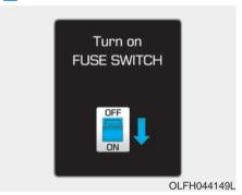
If the fuse switch is OFF, "Turn on FUSE SWITCH" message will appear.
