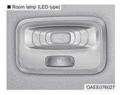
Your vehicle is equipped with LED lamps. LED lamps do not have replaceable bulbs. If the LED lamp does not operate, have the vehicle checked by an authorized HYUNDAI dealer.
