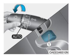
Adaptive front lighting system uses the steering angle and vehicle speed, to keep your field of vision wide by swiveling and leveling the headlamp. Change the switch to the AUTO position when the vehicle is in the ready ( ) mode. The adaptive front lighting system will operate when the headlamp is ON. To turn off the AFLS, change the switch to other positions. After turning the AFLS off, headlamp swiveling no longer occurs, but leveling operates continuously.
