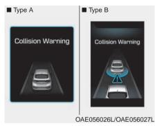
This warning message appears on the LCD display with a warning chime.
