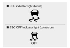
When the Engine Start/Stop button is placed to the ON position, the ESC indicator light illuminates, then goes off if the ESC system is operating normally.
