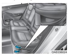
The high voltage battery cooling duct is located on the left side of the rear seats. The cooling duct cools down the high voltage battery.
