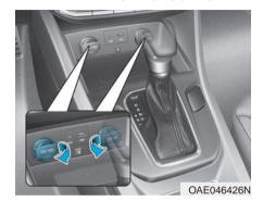
The power outlet is designed to provide power for mobile telephones or other devices designed to operate with vehicle electrical systems. The devices should draw less than 180 W (Watts) with the vehicle in the ready ( ) mode.
