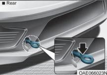
If towing is necessary, we recommend you to have it done by an authorized HYUNDAI dealer or a commercial tow truck service. If towing service is not available in an emergency, your vehicle may be temporarily towed using a cable or chain secured to the emergency towing hook at the rear of the vehicle.
