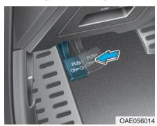
Check whether the stroke is within specification when the parking brake pedal is depressed with 44 lb (20 kg, 196 N) of force. Also, the parking brake alone should securely hold the vehicle on a fairly steep grade. If the stroke is more or less than specified, have the parking brake adjusted by an authorized HYUNDAI dealer.
