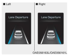
A visual warning appears on the cluster LCD display. Either the left lane line or the right lane line in the cluster LCD display will blink depending on which direction the vehicle is veering.
