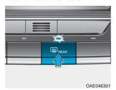
The defroster heats the window to remove frost, fog and thin ice from the interior and exterior of the rear window while the vehicle is in the ready ( ) mode.
