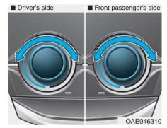
Turn the knob to the right to increase the fan temperature and airflow. Turn the knob to the left to decrease fan temperature.
