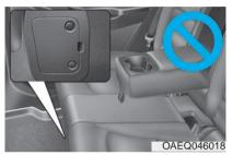
Never touch the safety plug. The safety plug is attached to high voltage hybrid battery system. Touching the safety plug will result in death or serious injury.
