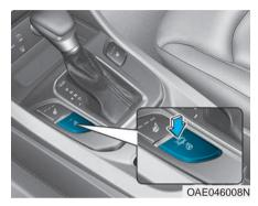
When the Engine Start/Stop button is in the ON position or when the vehicle is in the ready ( ) mode, press the heated steering wheel button to warm the steering wheel. The indicator on the button will illuminate. To turn the heated steering wheel off,
