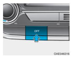
Push the OFF button to turn off the air climate control system. You can still operate the mode and air intake buttons as long as the Engine Start/ Stop button is in the ON position.
