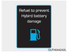
This warning message is displayed when the fuel tank is nearly empty.
