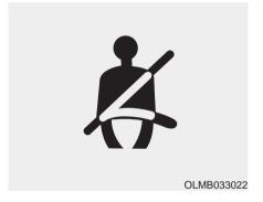
As a reminder to the driver, the seat belt warning light will illuminate and warning chime will sound for approximately 6 seconds each time you place the Engine Start/Stop button to the ON position if the seat belt is unfastened.
