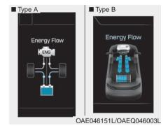
The engine braking is simultaneously used to decelerate the vehicle and to charge up the high-voltage battery.
