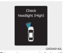
This warning message is displayed if the headlamps are not operating properly. The headlamp bulb may need to be replaced.
