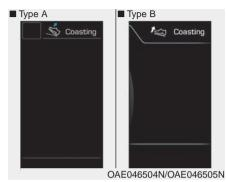
A chime will sound and the coasting guide indicator will blink four times to inform the driver when to take the foot off from the accelerator by anticipating a decelerating event\* based on the analysis of driving routes and road conditions of the navigation. It encourages the driver to remove foot from the pedal and allow coasting down the road with EV motor only. This helps prevent unnecessary fuel consumption and increases fuel efficiency.
