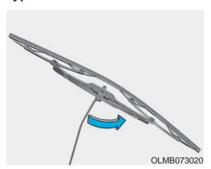
1. Raise the wiper arm and slightly rotate the wiper blade assembly to expose the plastic locking clip.
