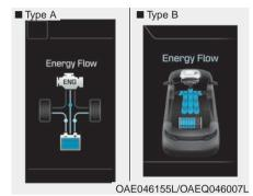
The engine and regenerative brake system charges up the high-voltage battery.
