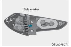
Remove the socket from the assembly by turning the socket counterclockwise until the tabs on the socket align with the slots on the assembly.
