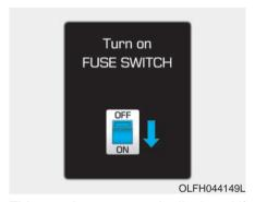
This warning message is displayed if the fuse switch located on the fuse box under the steering wheel is OFF. You should turn the fuse switch on.
