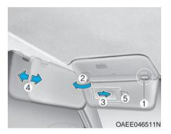
To use a sunvisor, pull it downward. To use a sunvisor for a side window, pull it downward, unsnap it from the bracket (1) and swing it to the side (2). To use the vanity mirror, pull down the sunvisor and slide the mirror cover (3). Adjust the sunvisor forward or backward (4) as needed (if equipped). Use the ticket holder (5) to hold tickets (if equipped).
