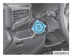
Detach the speed restriction label from the sealant bottle, and place it in a highly visible place inside the vehicle such as on the steering wheel to remind the driver not to drive too fast.
