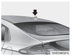
The shark fin antenna will receive the transmit data (example: AM/FM, SXM signal, GPS).
