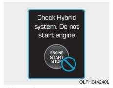
This warning message is displayed when the hybrid battery power (SOC) level is low. A warning chime will sound until the problem is solved. In this case have your vehicle inspected by an authorized HYUNDAI dealer.
