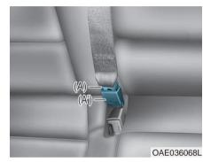
Insert the tongue plate (A) into the buckle (A') until an audible "click" is heard, indicating the latch is locked. Make sure the belt is not twisted.
