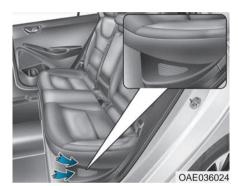
The high-voltage battery cooling duct is located on the left side of the rear seats. The cooling duct cools down the high-voltage battery. When the high-voltage battery cooling duct is blocked, the high-voltage battery may be overheated and the vehicle performance may become limited and set a hybrid warning lamp. Do not obstruct the cooling duct with any other objects.
