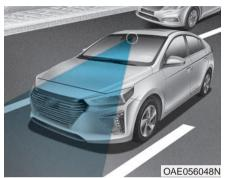
This Lane Departure Warning System detects the lane with the sensor at the front windshield and warns you when your vehicle leaves the lane.
