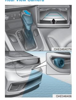
The Rear View Camera will activate when the vehicle is in the ready () mode and when you shift to the R (Reverse) position.
