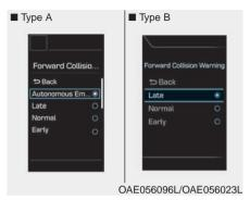
The driver can select the initial warning activation time on the LCD display. Go to the 'User Settings  $\rightarrow$  Driving Assist  $\rightarrow$  FCW (Fwd. Collision Warning)  $\rightarrow$  Late/Normal/Early'.
