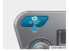
If you press the DRIVER ONLY button(\$\mathbf{s}^{DRIVER}\_{ONLY}) and the indicator light illuminates, air mostly blows in the direction of the driver's seat.
