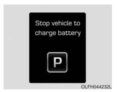
This warning message is displayed when the hybrid battery power (SOC) level is low.
