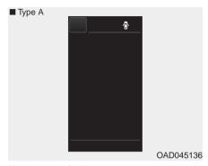
If the door/tailgate open warning is blocked with another warning message, an icon will appear on the top of the LCD display.
