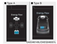
The hybrid system informs the drivers its energy flow in various operating modes. While driving, the current energy flow is specified in 11 modes. For more information, refer to HEV Energy Flow in the "Hybrid System Overview" provided in front of the owner's manual.
