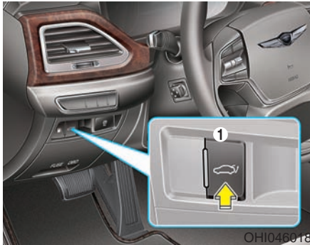
(2) Power Trunk Open button
