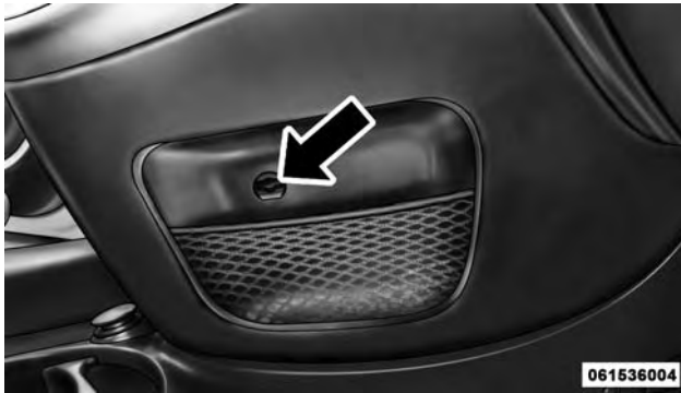
Gear Selector Override Access Hole
