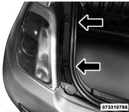
Tail Lamp Assembly Screws
