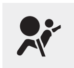
SRS warning light
