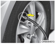
4. Unscrew the valve cap from the valve of the defective wheel and screw filling hose (2) of the sealant bottle onto the valve.
