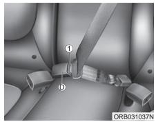
To unfasten the rear center belt Press the release button (1) on the buckle (D) and remove the tongue plate from the buckle (D).
