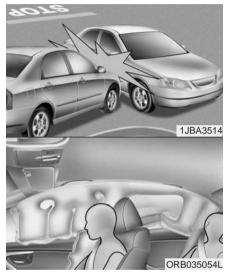
Although the driver's and front passenger's air bags are designed to inflate only in frontal collisions, they also may inflate in other types of collisions if the front impact sensors detect a sufficient impact. Side impact air bags and curtain air bags are designed to inflate only in side impact collisions or rollover situations, but they may inflate in other collisions if the side impact sensors detect a sufficient impact.
