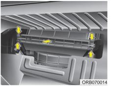
3. Remove the climate control air filter cover while pressing the lock of the cover.
