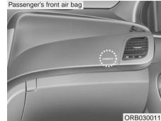
The purpose of the SRS is to provide the vehicle's driver and/or the front passenger with additional protection than that offered by the seat belt system alone in case of a frontal impact of sufficient severity. The SRS uses sensors to gather information about the driver's seat position, the driver's and front passenger's seat belt usage and impact severity.
