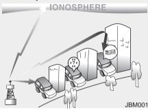
AM and FM radio signals are broadcast from transmitter towers located around your city. They are intercepted by the radio antenna on your vehicle. This signal is then processed by the radio and sent to your vehicle speakers.
