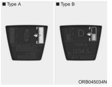
WARNING - Fuel gauge Running out of fuel can expose vehicle occupants to danger. You must stop and obtain additional fuel as soon as possible after the warning light comes on or when the gauge indicator comes close to the E level.
