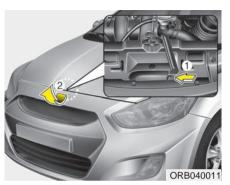
Go to the front of the vehicle, raise the hood slightly, push the secondary latch (1) to the left and lift the hood (2).
