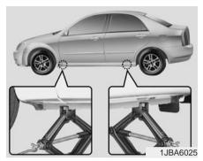
7. Place the jack at the front or rear jacking position closest to the tire you are changing. Place the jack at the designated locations under the frame.
