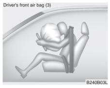
A fully inflated air bag, in combination with a properly worn seat belt, slows the driver's or the passenger's forward motion, reducing the risk of head and chest injury.
