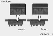
A vehicle's electrical system is protected from electrical overload damage by fuses. This vehicle has 2 fuse panels, one located in the driver's side panel bolster, the other in the engine compartment. If any of your vehicle's lights, accessories, or controls do not work, check the appropriate circuit fuse. If a fuse has blown, the element inside the fuse will be melted.
