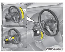
To change the steering wheel angle and height, pull down the lock release lever (1), adjust the steering wheel to the desired angle (2) and height (3), then pull up the lock-release lever to lock the steering wheel in place. Be sure to adjust the steering wheel to the desired position before driving.
