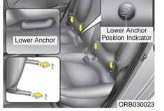
Child restraint symbols are located on the left and right rear seat backs to indicate the position of the lower anchors for child restraints
