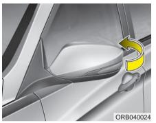
*Folding the side view mirror (if equipped)* To fold side view mirror, grasp the housing of mirror and then fold it toward the rear of the vehicle.
