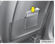
Seatback pocket (if equipped) The seatback pocket is provided on the back of the front passenger's and driver's seatbacks.
