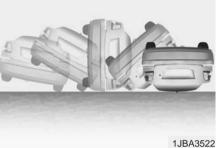
· Front air bags may not inflate in rollover accidents because air bag deployment would not provide additional protection to the occupants.
