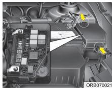
After checking the fuse panel in the engine compartment, securely install the fuse panel cover. If not, electrical failures may occur from water contact.
