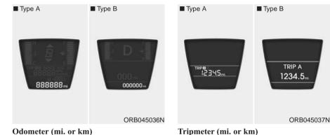
The odometer indicates the total distance the vehicle has been driven.
