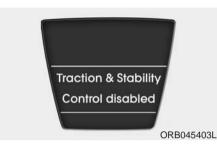
Press the ESC OFF button for more than 3 seconds. ESC OFF indicator light and message illuminates and ESC OFF warning chime will sound. At this state, the engine control function and brake control function does not operate. In other words, the vehicle stability control function does not operate any more.
