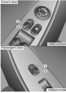
With central door lock switch (if equipped)
