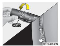
Auto light position (if equipped) When the light switch is in the AUTO light position, the taillights and headlights will turn ON or OFF automatically depending on the amount of light outside the vehicle.
