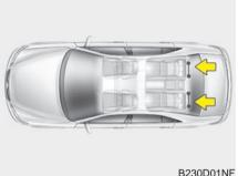
Securing a child restraint seat with child seat lower anchor system
