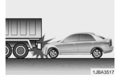
· Just before impact, drivers often brake heavily. Such heavy braking lowers the front portion of the vehicle causing it to "ride" under a vehicle with a higher ground clearance. Air bags may not inflate in this "under-ride" situation because deceleration forces that are detected by sensors may be significantly reduced by such "under-ride" collisions.
