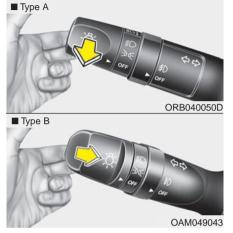
To flash the headlights, pull the lever towards you. It will return to the normal (low beam) position when released. The headlight switch does not need to be on to use this flashing feature.
