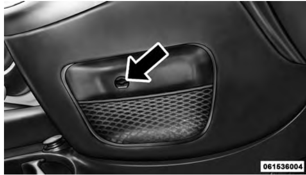
Gear Selector Override Access Hole
