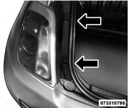
Tail Lamp Assembly Screws
