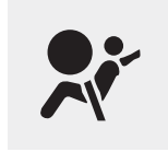
SRS warning light
