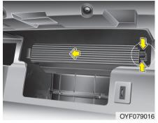
3. Remove the climate control air filter cover while pressing the lock on the right of the cover.
