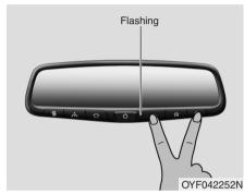
1. For first-time programming, press and hold the two outside buttons ( , ), ), HomeLink® Channel 1 and Channel 3, until the indicator light begins to flash (after 10 seconds). Release both buttons. Do not hold the buttons for longer than 20 seconds.
