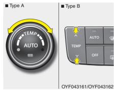
2. Turn the temperature control knob or button to set the desired temperature.
