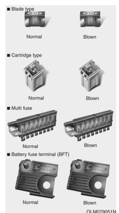
A vehicle's electrical system is protected from electrical overload damage by fuses. This vehicle has 2 fuse panels, one located in the driver's side panel bolster, the other in the engine compartment.
