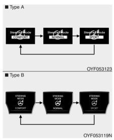
When steering mode button is pressed, steering mode will display as shown for 4 seconds.
