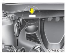
The refrigerant label is located on the engine block as shown in the drawing. The label contains the following information:
