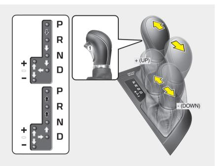
Depress the brake pedal and the lock release button (1) when shifting, if your vehicle is equipped shift lock system.
