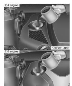
If it is near or at L, add enough oil to bring the level to F. **Do not overfill.**
