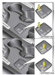
Type C (with air ventilation) (for driver's seat, if equipped)
