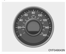
The speedometer indicates the speed of the vehicle.
