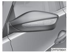
Side repeater light bulb replacement (if equipped)
