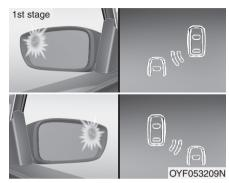
If a vehicle is detected within the boundary of the system, a yellow warning light will illuminate inside of the outside rearview mirror glass.
