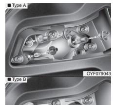
Remove the socket from the assembly by turning the socket counterclockwise until the tabs on the socket align with the slots on the assembly.
