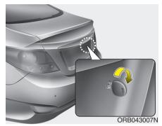
**Opening the trunk** *With the key* To open the trunk, insert the key and turn it clockwise.
