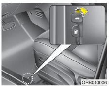
*With the trunk lid release lever* To open the trunk from inside the vehicle, pull up the trunk lid release lever.
