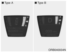
A WARNING - Fuel gauge Running out of fuel can expose vehicle occupants to danger. You must stop and obtain additional fuel as soon as possible after the warning light comes on or when the gauge indicator comes close to the E level.
