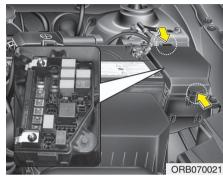
After checking the fuse panel in the engine compartment, securely install the fuse panel cover. If not, electrical failures may occur from water contact.
