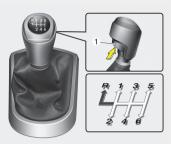
The shift lever can be moved into any of the forward gears without pressing the button (1).
