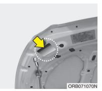
The refrigerant label is located on the underside of the hood.
