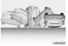
Front air bags do not inflate in rollover accidents. However, side impact and curtain air bags may inflate in a rollover, when it is detected by the rollover sensor.
