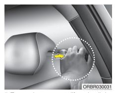
5. To use the rear seat, lift and pull the seatback backward. Push the seatback firmly until it clicks into place. Make sure the seatback is locked in place. When you return the seatback to its upright position, always be sure it has locked into position by pushing on the top of the seatback.
