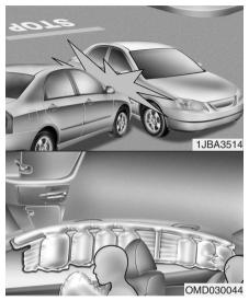
Although the front air bags (driver's and front passenger's air bags) are designed to inflate only in frontal collisions, they also may inflate in other types of collisions if the front impact sensors detect a sufficient impact. Side impact and curtain air bags are designed to inflate only in side impact collisions, but they may inflate in other collisions if the side impact sensors detect a sufficient impact.
