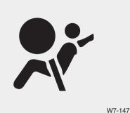
When the ignition switch is turned ON, the indicator light should illuminate for approximately 6 seconds, then go off. Have the system checked if:
