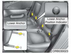
Child restraint symbols are located on the left and right rear seat backs to indicate the position of the lower anchors for child restraints
