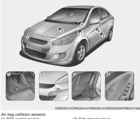
(1) SRS control module(2) Front impact sensor
