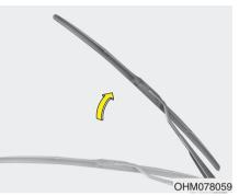
*Front windshield wiper blade* Type B 1. Raise the wiper arm.
