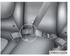
Pull and insert the tongue plate (C) into the open end of the buckle (D) until an audible "click" is heard, indicating the latch is locked.
