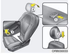
**Reinstall** To reinstall the headrest:
