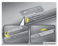
2. Rotate the cover half way and insert the cover on the roof hole as the illustration.
