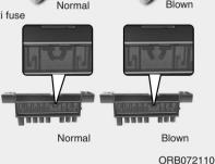
A vehicle's electrical system is protected from electrical overload damage by fuses. This vehicle has 2 fuse panels, one located in the driver's side panel bolster, the other in the engine compartment.
