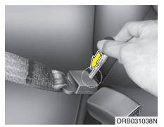
To disconnect the rear center belt Insert a key or narrow-ended tool into the groove located on buckle.
