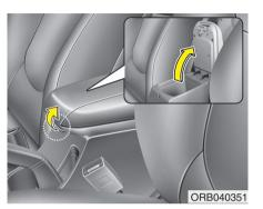
**Center console storage** To open the center console storage, pull up the lever.
