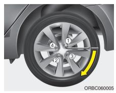
Then position the wrench as shown in the drawing and tighten the wheel nuts. Be sure the socket is seated completely over the nut. Do not stand on the wrench handle or use an extension pipe over the wrench handle. Go around the wheel tightening every other nut until they are all tight. Then double-check each nut for tightness. After changing wheels, have an authorized HYUNDAI dealer tighten the wheel nuts to their proper torgue as soon as possible.
