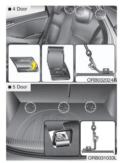
Securing a child restraint seat with "Tether Anchor" system Child restraint hook holders are located on the package tray or on the floor behind the rear seats.
