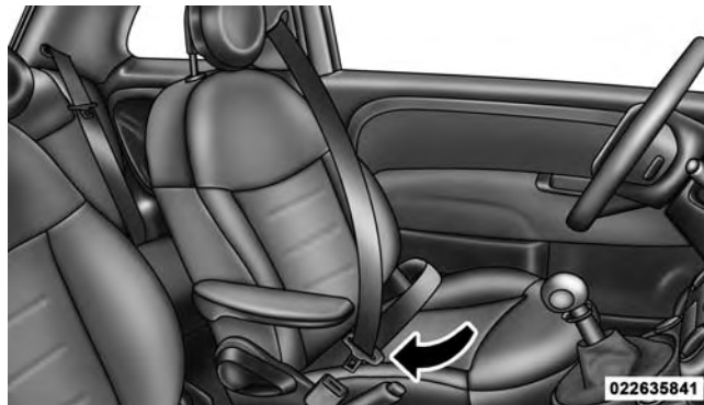
Inserting Latch Plate Into Buckle
