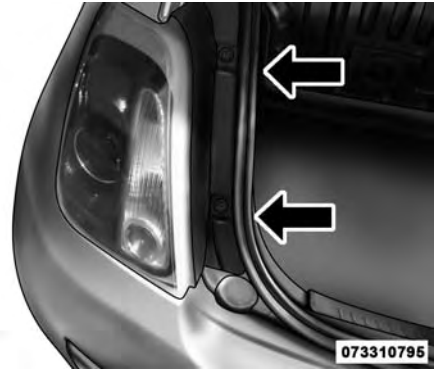
Tail Lamp Assembly Screws
