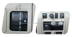
While the light switch is on, rotate the dial downward to dim the instrument panel illumination. Rotate the dial upward to make the illumination brighter. When the dial is fully rotated upward, the instrument panel illumination becomes full bright.
