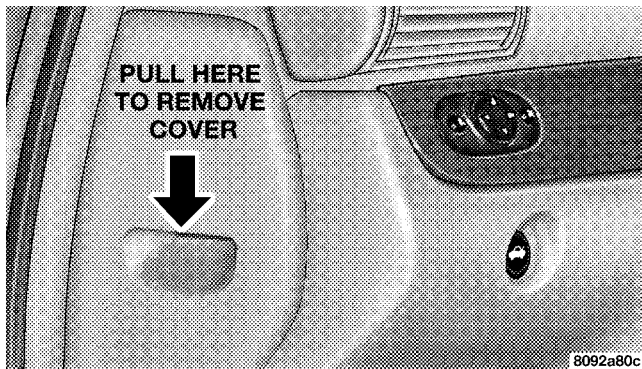
Fuse Panel Cover
