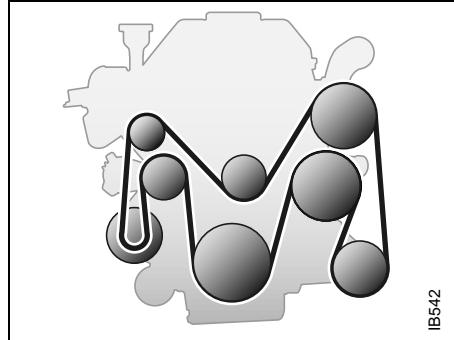
Routing of the Poly-V-belt: 4-cylinder engine
