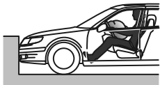
Sensor detects deceleration and sends a signal via the control module to a gas generator that inflates the airbag.
