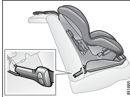
Semi-rigid 2-point lower attachment with top tether
