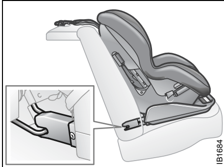
Rigid 2-point lower attachment with top tether
