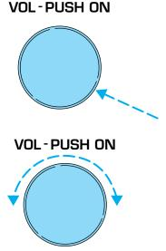
If the volume is set above a certain level and the ignition is turned off, the volume will come back on at a "nominal" listening level when the ignition switch is turned back on.
