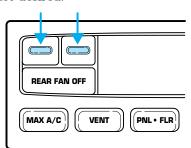
For continuous maximum cooling, push the blue button until 16°C (60°F) is shown in the display window. The EATC will continue maximum cooling (disregarding the displayed temperature) until a warmer temperature is selected by pressing the red button.
