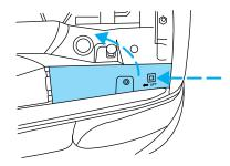
2. Disconnect the electrical connector from the bulb by pulling rearward.
