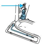
7. Position the jack according to the following guides and turn the jack handle clockwise until the tire is a maximum of  $25~\mathrm{mm}$  (1 inch) off the ground.
