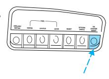
five seconds. After a successful reset, the message center will display OIL LIFE RESET TO 100%. (If you have established a personalized oil reset percentage, the display will show that percentage instead of 100%.) This reset procedure should be performed only after an oil change to ensure accurate oil life indications.
