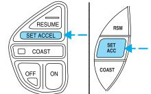
Accelerate with your accelerator pedal. When the desired vehicle speed is reached, press and release SET/SET ACC/SET ACCEL.
