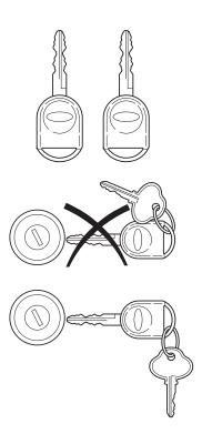
momentary concern if they are too close to the key during engine start. If a problem occurs, turn ignition OFF and restart the engine with all other objects on the key ring held away from the ignition key. Check to make sure the encoded ignition key is an approved Ford encoded ignition key.
