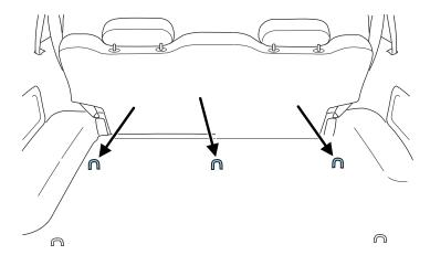
3. Locate the correct anchor for the selected rear seating position. The anchors must remain accessible. Make sure the anchors are not covered by the cargo mat or other objects.
