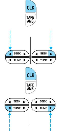
The CLK control will allow you to switch between media display mode (radio station, stereo information, etc.) and clock display mode (time).
