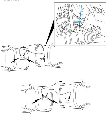
2. Remove the jumper cable on the negative (-) connection of the booster vehicle's battery.
