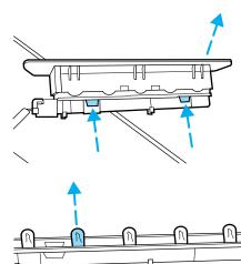
4. Pull the bulb straight out of the socket and push in the new bulb.
