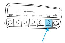
The engine oil life left has two phases. The first display will indicate the oil change status (OK, SOON, REQUIRED). The second display will indicate the percentage of oil life remaining. The display OIL TEMP SIGNAL ERROR indicates a problem with the system. Following this display, contact your dealer or qualified service technician for system maintenance.
