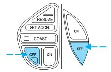
Once speed control is switched off, the previously programmed set speed will be erased.
