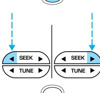
To set the minute, press and hold the CLK control and press TUNE:
