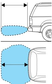
The reverse sensing system is automatically enabled when the gear selector is placed in R (Reverse) and the ignition is ON. A reverse sensing control allows the driver to disable the reverse sensing system only when the ignition is ON, and the gear selector is in R (Reverse).
