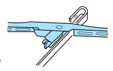
3. Attach the new wiper to the wiper arm and press it into place until a click is heard.
