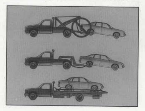
Before hooking up to a tow truck, be sure to read all the information in "Towing Your Vehicle" earlier in this section. Also be sure to use the proper hook-up for your particular vehicle.
