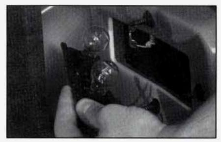
Carefully push one end of the plastic taillamp brace in while pulling the brace toward the front of the vehicle.
