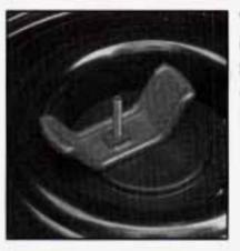
Turn the wing nut counterclockwise and remove it. Then lift off the adapter and remove the spare tire.
