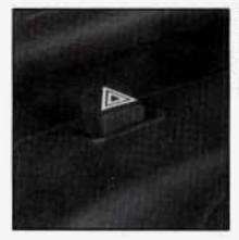
Press the switch to make your front and rear turn signal lamps flash on and off.
