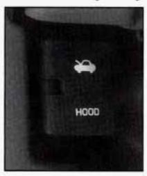
To open the hood, first pull the handle inside the vehicle. It is located in the area to the left and beneath the instrument panel.
