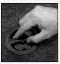
The equipment you'll need is in the trunk. Pull the carpeting from the floor of the trunk. Turn the center retainer nut on the compact spare tire housing counterclockwise to remove it.
