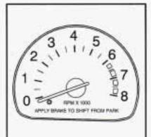
The tachometer tells you how fast the engine is running. It displays engine speed in hundreds of revolutions per minute (rpm).
