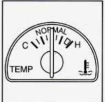
This gage shows the engine coolant temperature. If the gage pointer moves into the red area, your engine is too hot!
