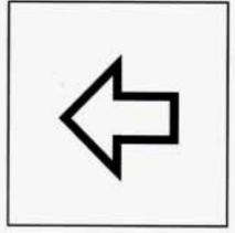
A green arrow on the instrument panel will flash in the direction of the turn or lane change. To signal a lane change, just raise or lower the lever until the arrow starts to flash. Hold it there until you complete your lane change. The lever will return by itself when you release it.
