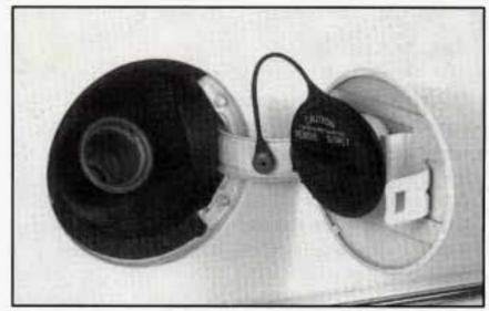
While refueling, hang the cap inside the fuel door. To take off the cap, turn it slowly to the left (counterclockwise).
