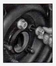
8. Replace the wheel nuts with the cone end of the nuts toward the wheel. Tighten each nut by hand or with the wheel wrench until the wheel is held against the hub.
