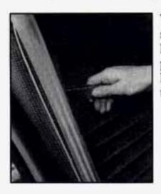
With the rear folding seatbacks, you can carry long cargo by folding down part or all of the rear seat. Pull this strap to fold down the seatback.
