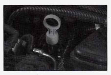
The automatic transaxle dipstick handle is red. Pull out the dipstick and wipe it with a clean rag or paper towel. Push it back in all the way, wait three seconds and then pull it back out again.
