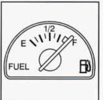
Your fuel gage shows how much fuel is in your tank. It works only when the engine is on. When the indicator nears EMPTY (E), you still have a little fuel left. You need to get more right away.
