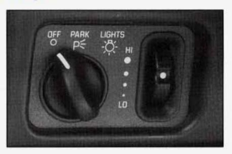
The headlamp switch is located on the left side of the instrument panel.
