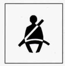
The safety belt light will also come on and stay on for about 20 seconds, then it will flash for about 55 seconds. If the driver's belt is already buckled, neither the chime nor the light will come on.
