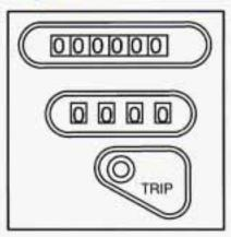
A trip odometer can tell you how many miles you have driven since you last set it to zero. To reset it, push the button.
