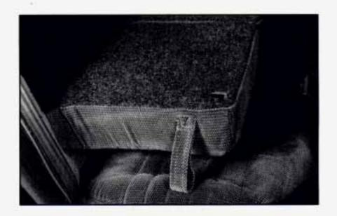
When you fold the seatback up, push the top of the seat, making sure the seat is completely closed to ensure the seat locks in a sudden stop or crash.
