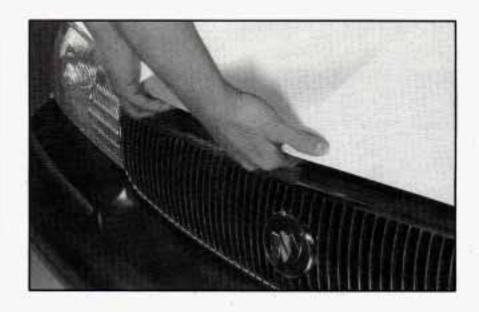
Then go to the front of the vehicle and release the secondary hood release, by moving the lever upward and to the right. Lift the hood.
