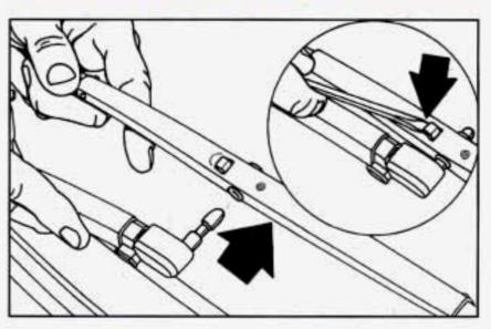
Replacement blades comes in different types and are removed in different ways. For proper blade size, see "Capacities and Specifications" in the Index. Here's how to remove the type with a release clip:
