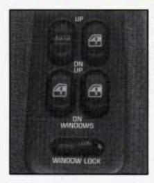
Switches on the driver's door armrest control each of the windows when the ignition is on. In addition, each passenger door has a switch for its own window.
