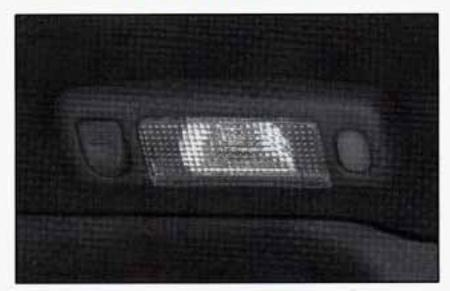
The rear seat reading lamps are turned on by pressing the switch next to the lamp above the rear doors. Press the switch again to turn the lamp off.
