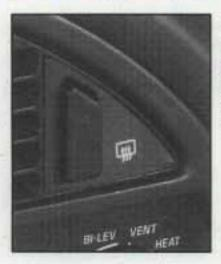
The lines you see on the rear window warm the glass. Press the button to start warming your window. Pressing the button again will shut it off.
