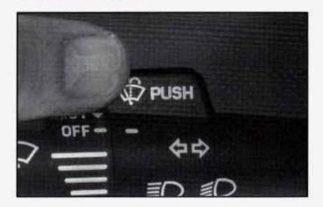
The top of the wiper lever has the word PUSH on it. To spray washer fluid on the windshield, press this portion of the lever towards the instrument panel.
