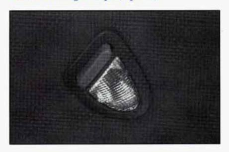
The front seat reading lamps are turned on by pressing the switch next to the lamp. Press the switch again to turn the lamp off.
