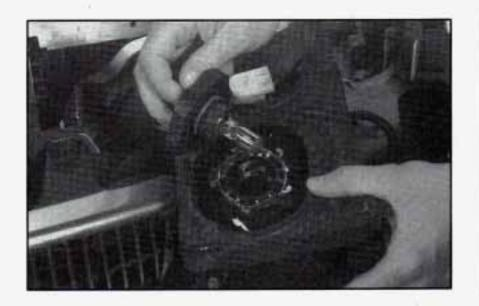
Pull the bulb/socket straight out from the access cover.
