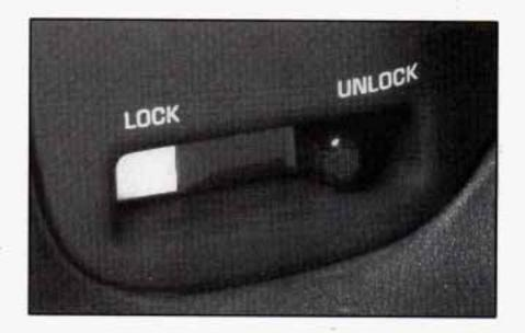
From the inside: To lock the door, slide the lock control rearward.
