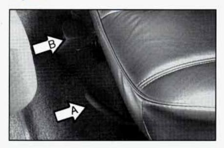
If you have this option, you have two levers under the front edge of the seat. The lever near the outer side of the seat (A) unlocks the seat allowing it to slide forward and back. The lever on the right (B) allows you to tilt the seat up and down.
