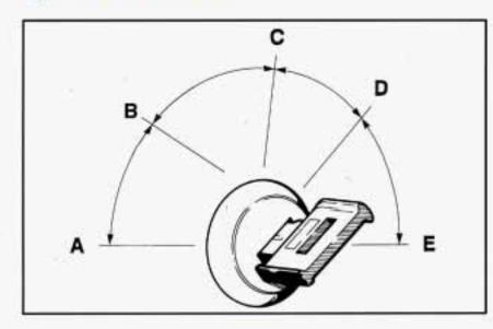
With the key in the ignition switch, you can turn the switch to five different positions:
