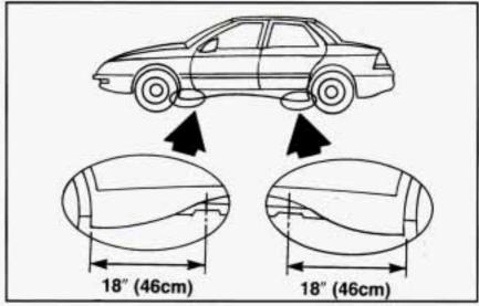
On some vehicles, a cover plate must be removed to find the wheel nuts. Carefully use the wedge end of the wheel wrench to pry it off. Be careful; the rim edges may be sharp. Don't try to remove it with your bare hands. Position the jack and raise the jack head until it fits firmly into the notch in the vehicle's frame nearest the flat tire. Put the compact spare tire near you.
