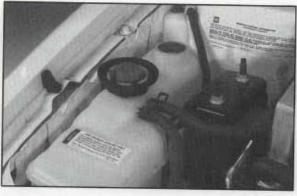
You can remove the coolant surge tank pressure cap when the cooling system, including the coolant surge tank pressure cap and upper radiator hose, is no longer hot. Turn the pressure cap slowly about one-quarter turn to the left and then stop.
