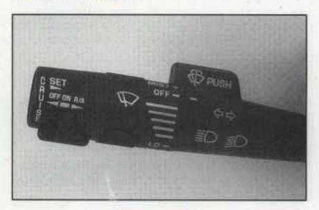
You control the windshield wipers by rotating the outer portion of the switch.
