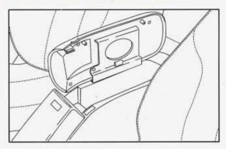
The armrest opens into a storage area for cassette tapes, gloves, etc. To open it, lift up on the driver's side front portion of the armrest. A tissue holder is located under the lid of the armrest.
