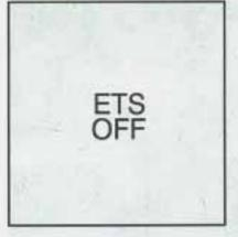
When the transaxle shift lever is in the THIRD (3) or OVERDRIVE (®) position and the parking brake is fully released, this warning light will come on to let you know if there's a problem with the system.
