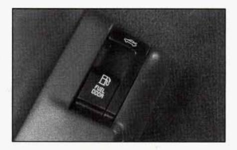
Pull up on the release lever to unlatch the fuel door. It is located on the floor to the left of the driver's seat.
