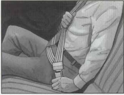
If the belt stops before it reaches the buckle, tilt the latch plate and keep pulling until you can buckle it. Pull up on the latch plate to make sure it is secure.
