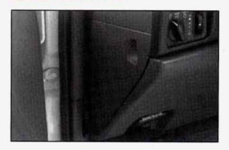
The main fuse panel is located on the left side of the instrument panel. To access the fuses, open the fuse panel door.
