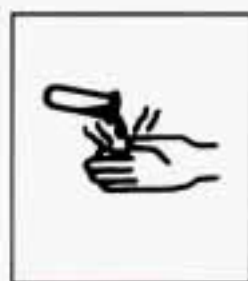
Caustic Battery Acid Could Cause Burns
