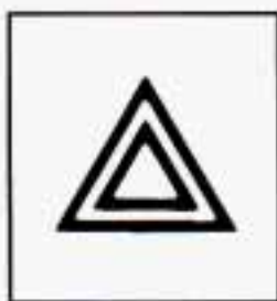
Hazard Warning Flasher
