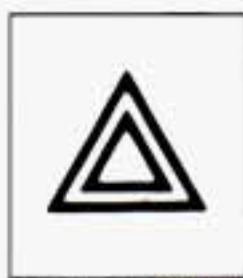
Hazard Warning Flasher
