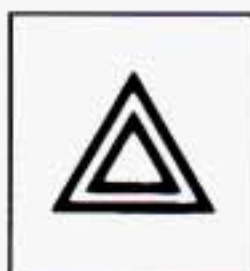
Hazard Warning Flasher
