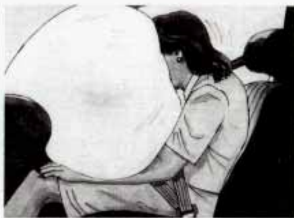
The right-front passenger's air bag is located in the instrument panel on the passenger's side.
