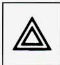
Hazard Warning Flasher
