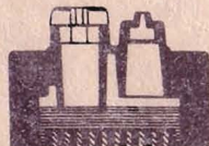
Remove cap from safety-vent and solution drops to correct level. Replace cap in filler hole.
