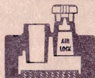
Place cap on safety-vent forming air lock in breather-chamber.
