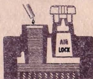
Fill well with distilled water. Air lock prevents solution rising above bottom of well.
