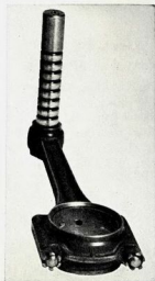
Fig. 6—Before Reaming the Split Type Pin Bushings They Must be Tightly Expanded into Rod With a Burnisher
