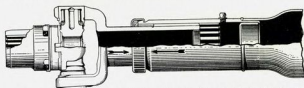
Fig. 44—Arrow on Universal Yoke of 1901 Must Align With Arrow on Propeller Shaft
