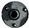
No. 10-24x5/8" flat head machine screw and wood grip nut. Window regulator to regulator board.
