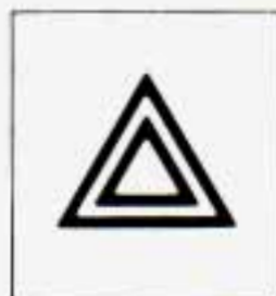
Hazard Warning Flasher
