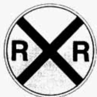
RAILROAD ADVANCE CROSSING
